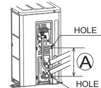
Run the connection cable to the rear of the outdoor unit within the A range of the arrows shown in the figure. (The switch cover becomes difficult to install.)
